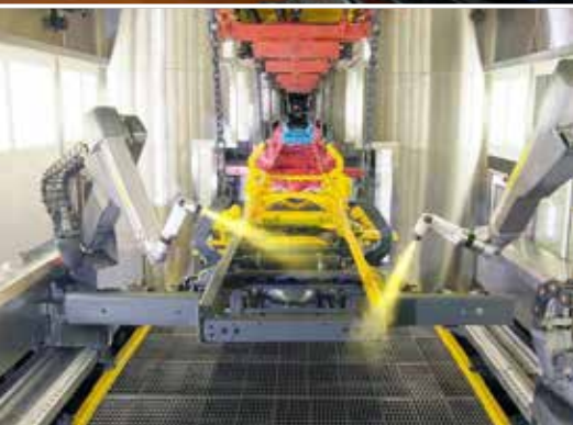
Leyland Trucks was the first truck plant in the world with a robotic chassis paint-spray shop on a moving production line. Meanwhile, other PACCAR factories acquired the concept.
