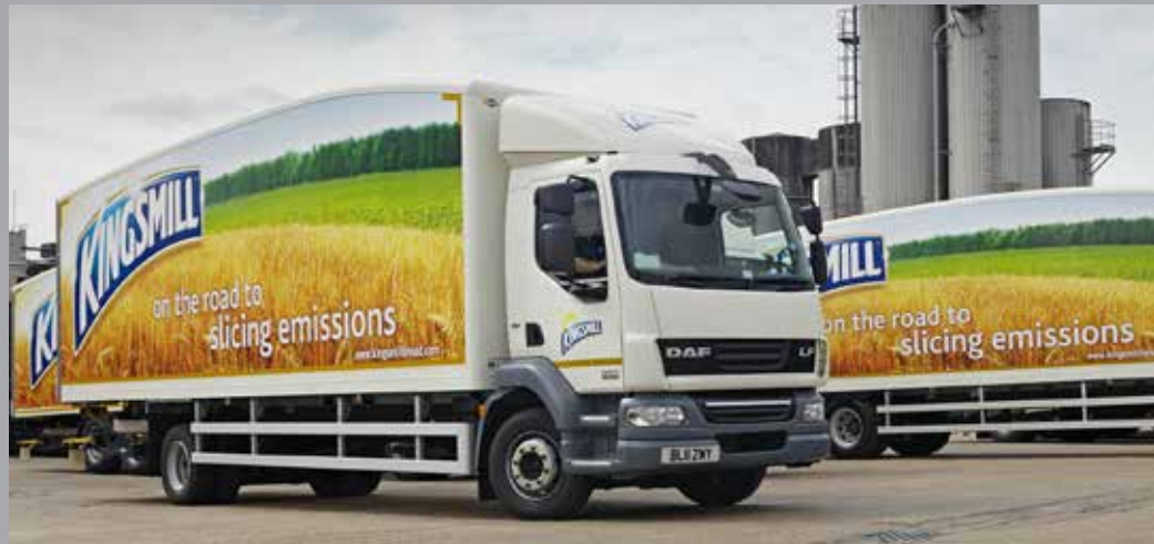
UK hauliers pay more for their diesel than anyone else, which explains this streamlined, fuel saving superstructure on this DAF LF.
